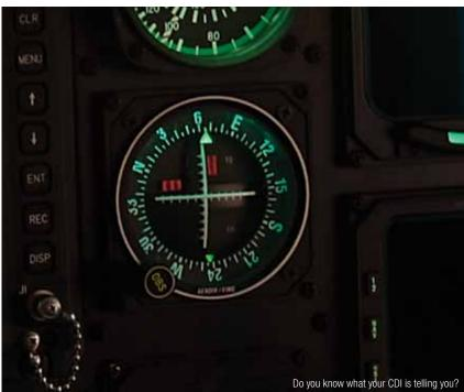
tional radio range — stations emit 360 radials, one for each degree of magnetic direction from the station.) The outside of the center circle actually represents the first two degrees of angular deviation, so "full-scale" deviation on either side of the center is 10 degrees.
