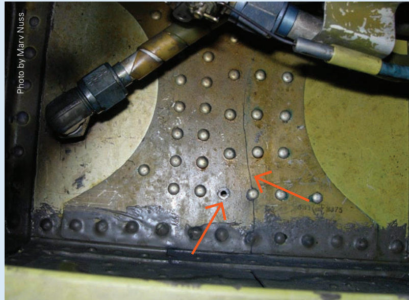
Fatigue induced auxiliary pump crack and popped rivet.
