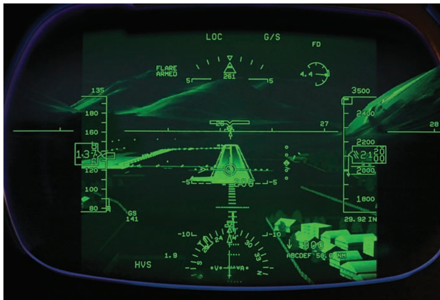
A HUD display of information from a Rockwell Collins EVS-3000 Enhanced Vision system.
