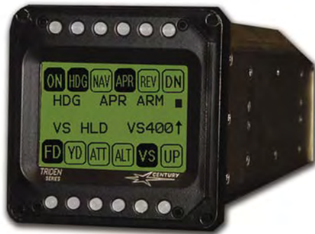
Figure 17-20. An example of an autopilot system.
