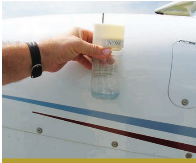
When checking fuel for contamination, always hold up against a contrasting object.
