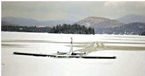
Snow bank related accidents are the greatest hazard to aircraft ground operations during the winter season.
