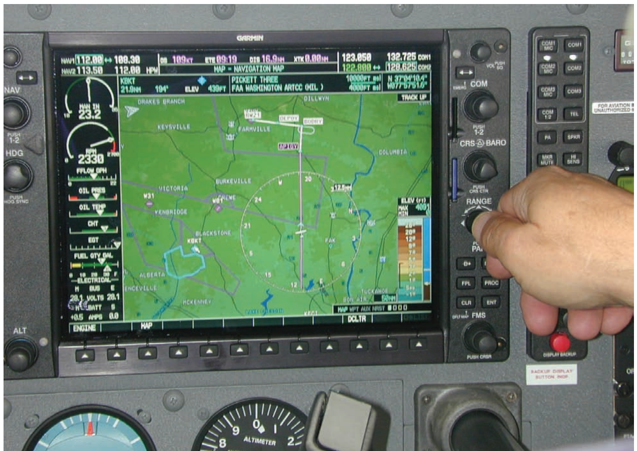
Never forget that the magenta line can guide you direct to anywhere ... including direct through regulatory, man-made, or natural obstacles.
