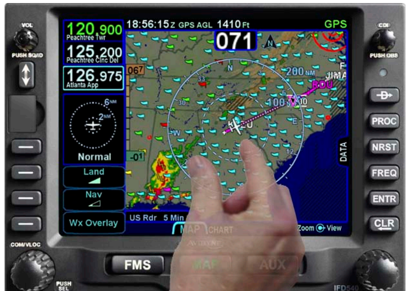
Onboard weather radar can help in making tactical decisions in flight.
