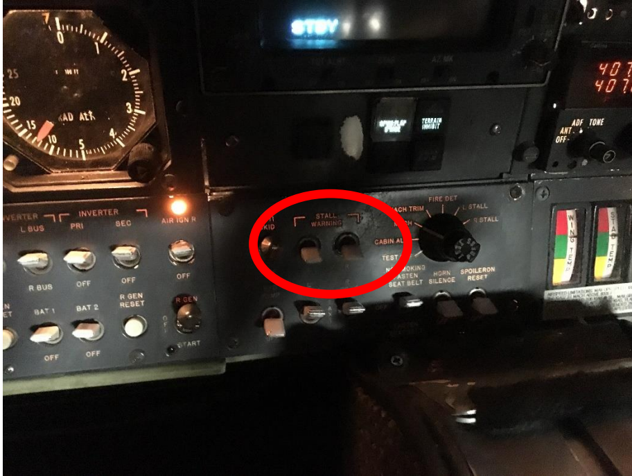
Photo 2: Lear 35A Stall Warning Switches on Captain's side forward instrument panel, indicated by red circle. 105
